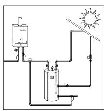
This system design demonstrates how to install a Bosch AquaStar 1600PS as part of a solar-based water heating system. Check your local codes to determine if you need a tempering valve.
